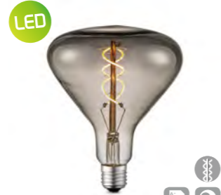
TLB-8020-06SM LED FLEX E27 2200K 6 W=15 W | 140 lm 25.000 hours CRI 80 Ø 14 CM ↓ 16.8 CM CERTIFICATE: DEKRA
